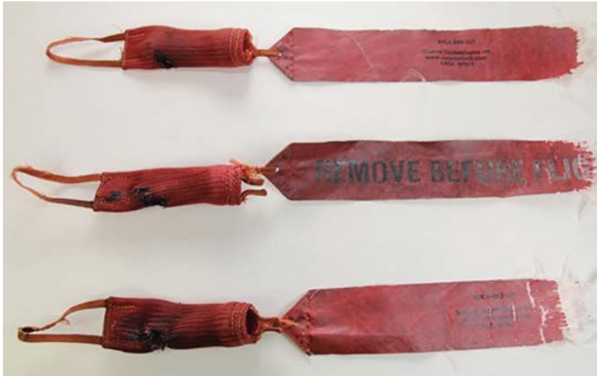
Figure 4: Pitot probe covers removed from 9M-MTK after the incident flight
