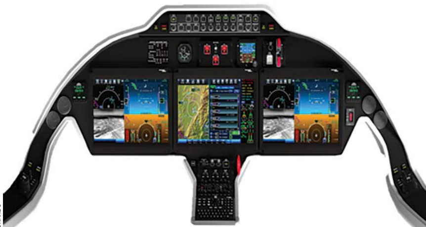
The AW609 will be equipped with a Collins Fusion avionics suite typical of business jets. It includes a sink-rate warning system and nacelle tilt-angle indicator.
