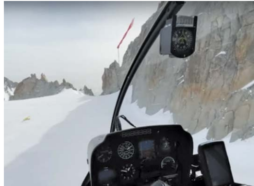
The behavior of the trim string is directly indicative of the airflow condition over the nose.
