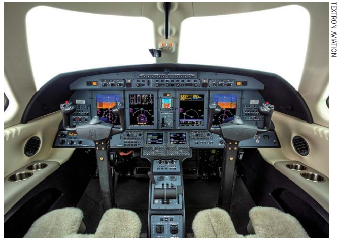
The Collins Pro Line 21 avionics suite of the Citation CJ4 Gen2.
